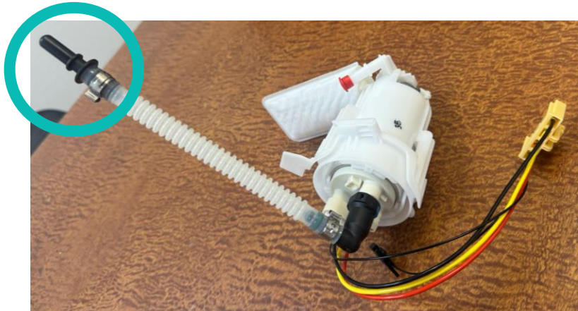
Fitting connected to the hose inside the tank
